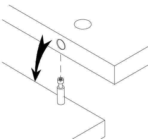
Now fit the hole in the edge of the joining board over the Cam Pin.
