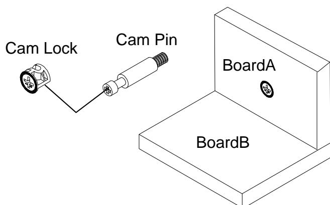
To assemble this product hardware called Cam Lock Fasteners are used. The below is information on how these work.
