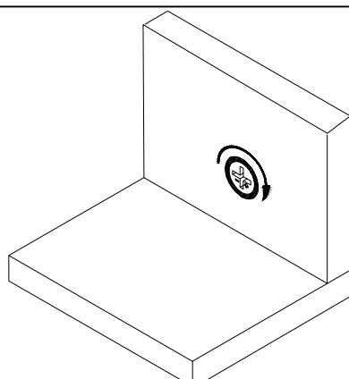
Use a Flat screwdriver to turn the Cam Lock clockwise one half turn so it locks onto the head of the Cam Pin. Turn only until it is snug. Over tightening could cause the Cam to bend or break. If it will not turn the full amount, turn the Cam Pin out (Counter-clockwise) one full turn, and try the Cam Lock again.
