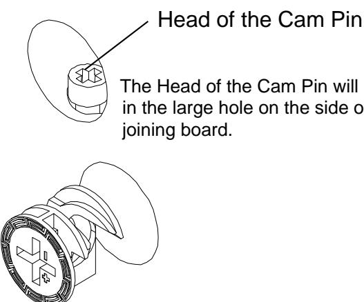
The Head of the Cam Pin will be visible in the large hole on the side of the joining board.
