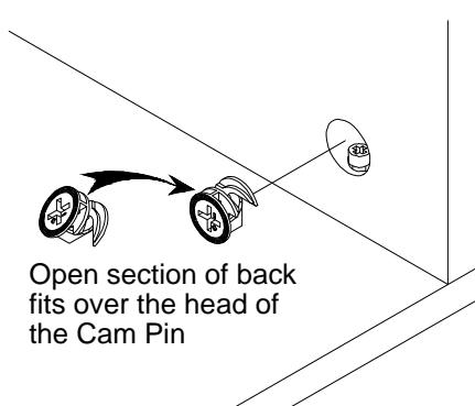
Open section of back fits over the head of the Cam Pin
